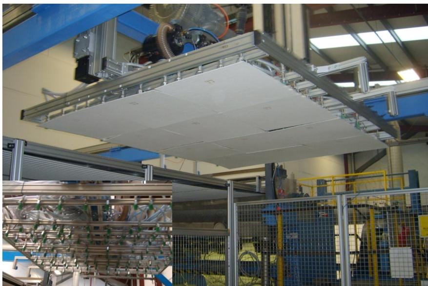
The main photograph above shows a series of 12 filter sheets being lifted pneumatically off the machine conveyor ready to be lowered onto a pallet. The photograph insert shows details of the PLC controlled pneumatic lifting system. A short video showing further detail of the new take-off system is available on request.
