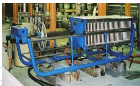
An Example of a Fully Refurbished 60cm Filter Press in action at Hydes Brewery Manchester, UK.
